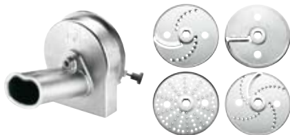
Vegetable cutter, stainless steel. 4 discs with 6 functions included: Slicing: 2 mm + 2.6 mm Shredding: 3 mm + 5 mm Rasping: 2 mm Julienne: 8x8 mm All dishwasher safe!
